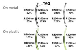
\* Read ranges are theoretical values that are calculated for non-reflective environment, in where antennas with optimum directivity are used with maximum allowed operating power according to ETSI EN 302 208 (2W ERP). Different surface materials may have an effect on performance.
